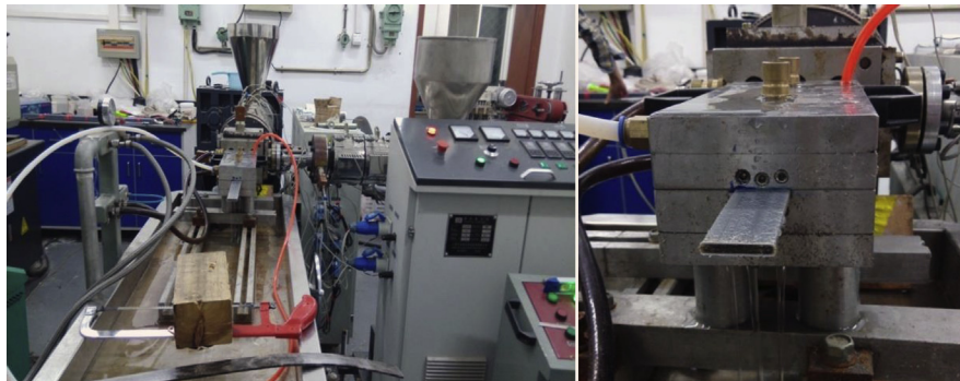
Figure 10.12 Production line of core-shell structured bamboo plastic composites
