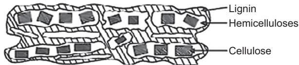
Figure 8.3 Structure organization of the three major constituents in the fibre cell wall (Kabir et al., 2012).
