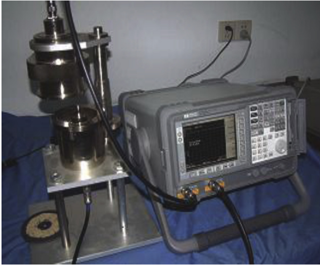
Figure 12.3 Setup for the electromagnetic shielding effectiveness test.
