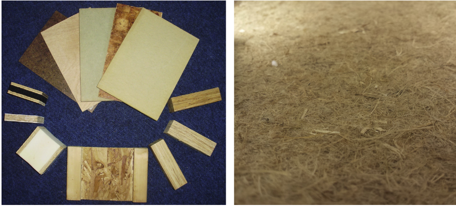
Figure 1.3 Various wood-based composites for construction (left = rigid composites and right = insulation mat).
