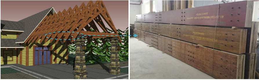
Figure 10.11 Large-span double beam component made by bamboo bundle wood hybrid laminated composites.
