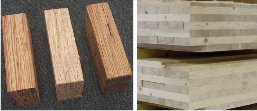
Figure 1.6 Consolidated composites: glulam and laminated veneer lumber (left) and cross-laminated lumber (right).
