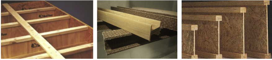
Figure 1.10 Various I-joists made of natural fibre composites (left = plywood flange, middle = long fibre hemp composite flange and right = oriented strand board flange).
