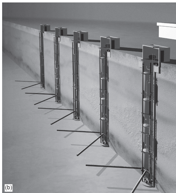
Fig. 10.3. (a) The SAFIRA test site at Bitterfeld with the five well shaft housings on the left-hand side and the on-site laboratory building on the right-hand side. (b) The well shafts and horizontal collection wells
