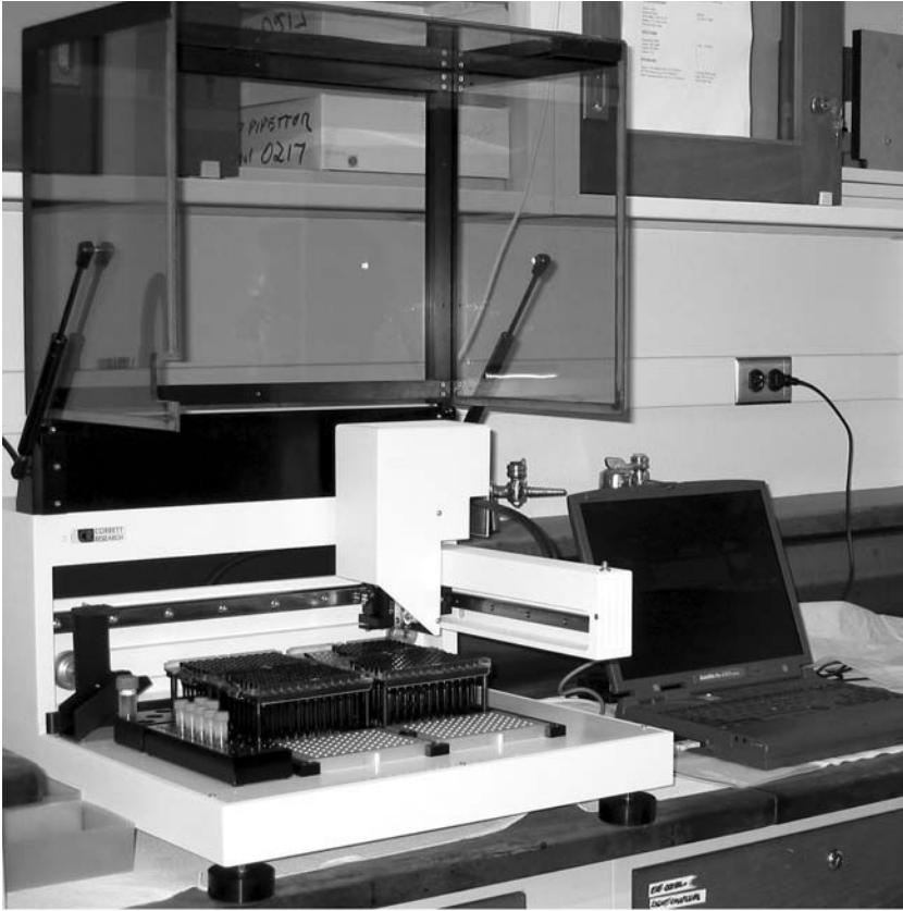
Fig. 5. The CAS-1200 pipetting robot (Corbett Research, Australia). The CAS-1200 is designed specifically for pipetting PCR reactions. The operating system for the robot is straightforward, easy to use, and runs in Windows XP. PCR reactions can be set up in 0.2-mL thin-walled PCR tubes with a 96-well or 384-well format.
