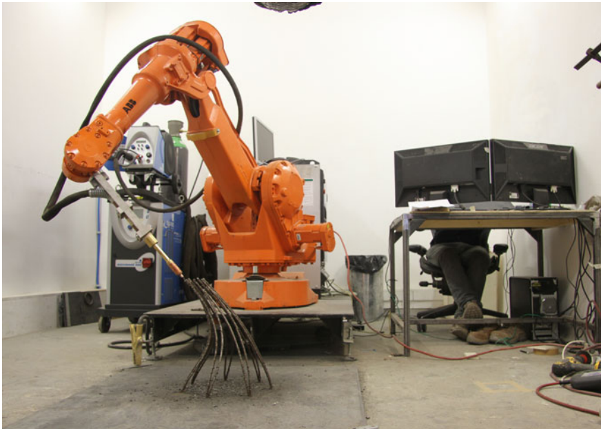
Fig. 3.35 The industrial robot is coupled with an advanced welding machine which can print with metals like stainless steel, aluminium, bronze or copper (Courtesy of Joris Laarman Lab)
