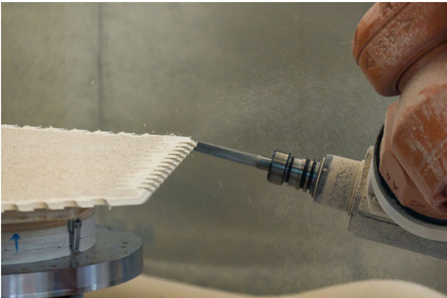
Fig. 3.22 Custom-made cutting and milling tools were installed on a seven-axis industrial robot (Courtesy of © ICD/ITKE University of Stuttgart)
