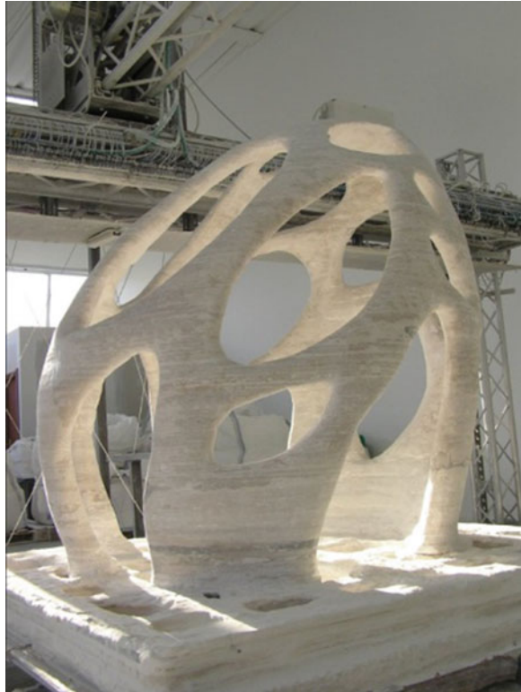
Fig. 3.25 D-Shape by Enrico Dini allows printing large-scale objects with the employment of a chemically refined sand as a binder (Courtesy of Enrico Dini)
