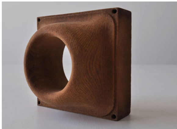
Fig. 3.27 Wood block designed by Anthony Giannini of Emerging Objects—an example of 3D printed wood as a possible building material obtained by waste (© Emerging Objects Corp.)
