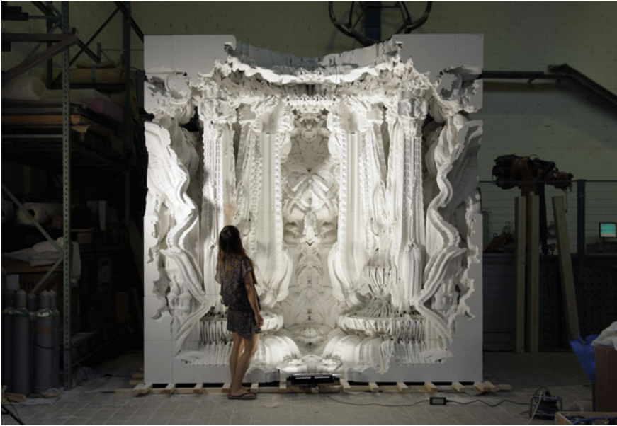
Fig. 4.48 Digital Grotto is a human scale 3D printed structure, detailed at the threshold of the human perception (Reproduced with permission of Michael Hansmeyer & Benjamin Dillenburger)
