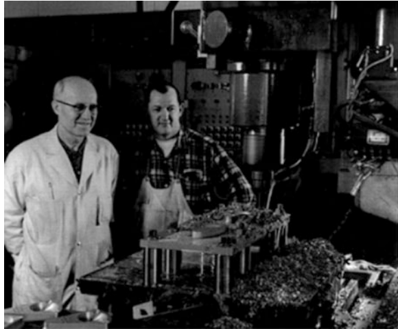
Fig. 3.1 Technicians observe the first Numerically Controlled milling machine at MIT (© 2014 Today's Machining World)
