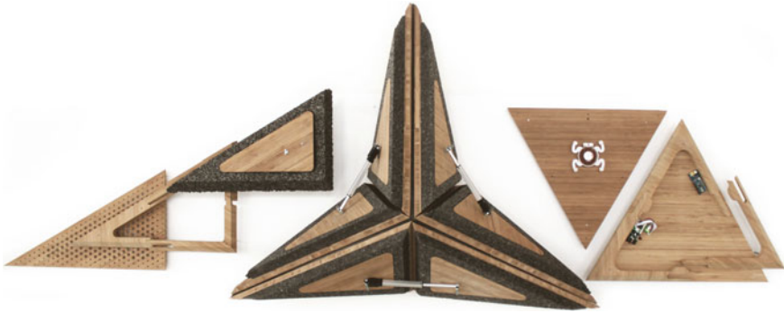
Fig. 4.55 The final result of the Resonant Chamber is achieved through fabricating component parts that could be assembled into a composite panel. By creating a face panel separate from the frame, each panel type could be uniformly bonded to the continuous membrane that comprises the hinge. A cap on the frame encloses either a DML exciter component, electronics controls or a solid reflective panel (Reproduced with permission of RVTR)
