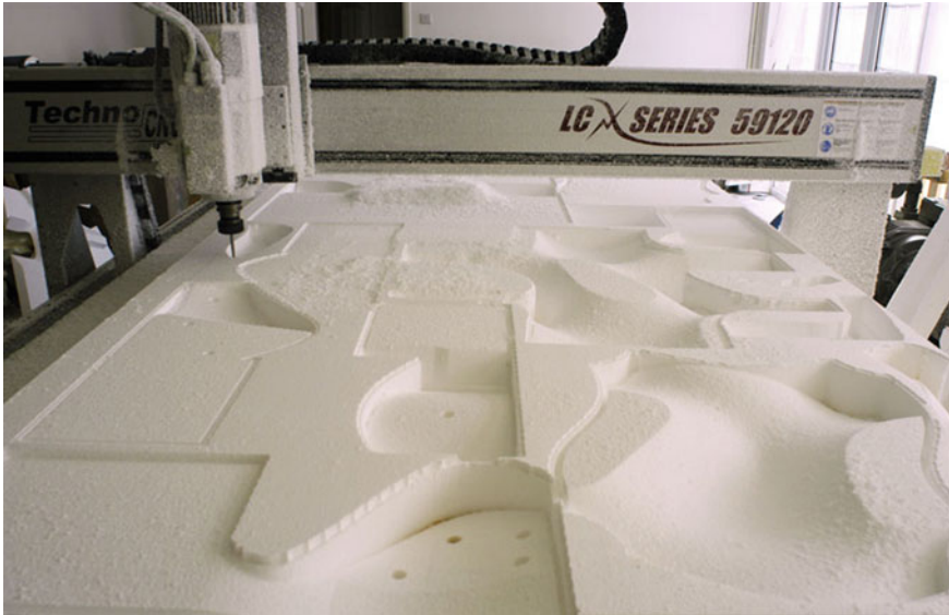
Fig. 3.3 CNC milling with a 3-axis milling machine (© 2010 MESA Studio)
