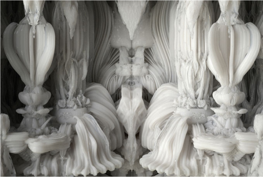
Fig. 4.50 The structure is made by a geometric mesh, containing 260 million highly detailed facets, that are individually defined through an algorithmic design and fabricated with 3D printing technology (Reproduced with permission of Michael Hansmeyer & Benjamin Dillenburger)
