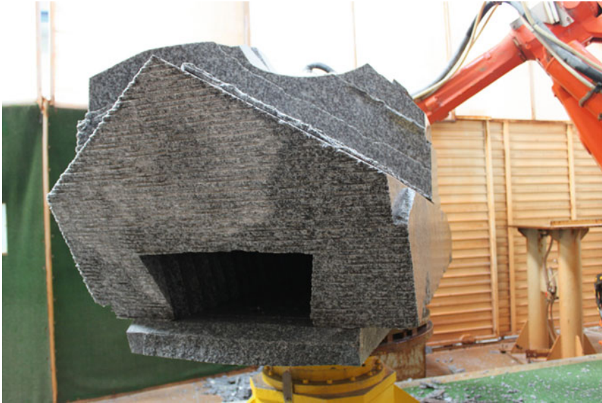
Fig. 3.23 Gaudi's Sagrada Familia. Mark Burry and his team turned to the robotically assisted methods for milling the granite blocks (© 2014 Royal Melbourne Institute of Technology)
