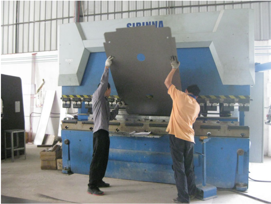
Fig. 3.5 CNC bending machine (© 2011 Jiangmen Dongji Metal Products Co.)
