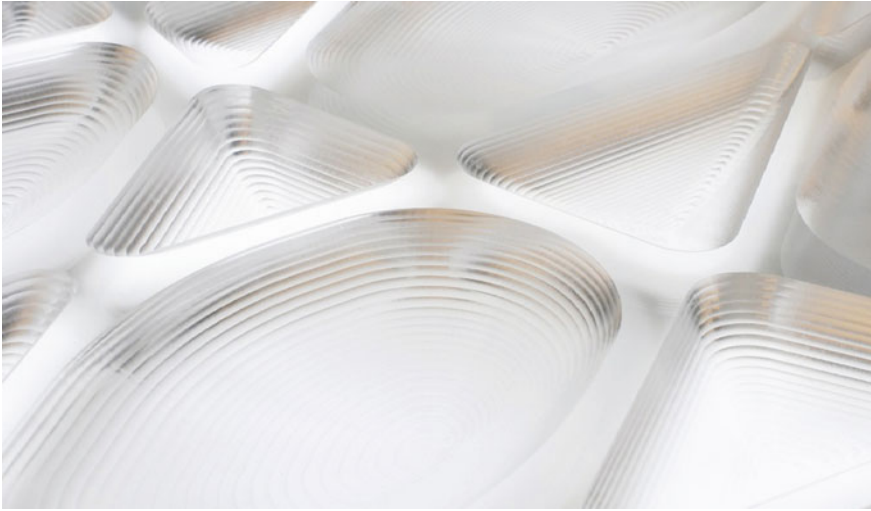
Fig. 4.60 Temporal Synapse, CNC milled acrylic sheet and cellular pattern detail (© 2009 PROJECTiONE LLC.)
