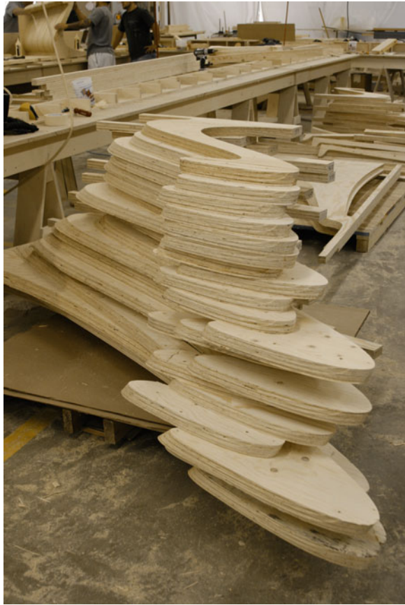
Fig. 4.47 Milled elements of the benches ready for assembly (Reproduced with permission of DECOI)
