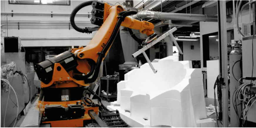
Fig. 3.17 A multi-axis CNC hotwire-cutter capable of processing four meters long EPS blocks was employed for the Periscope Tower (Courtesy of matter design)
