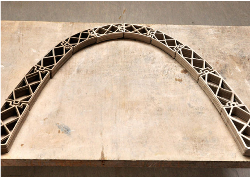
Fig. 4.33 The Interlocking Bricks assembled in a structural system (Reproduced with permission of Brian Peters)
