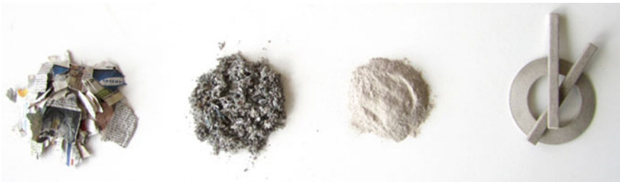
Fig. 3.29 Emerging Objects experiments with several material applications in additive manufacturing, focusing on the idea of reusing waste. Pictured above, recycled paper employed for 3D printing a house (© Emerging Objects Corp.)
