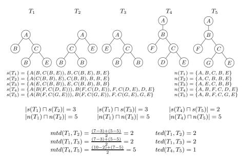
**Fig. 1.** This example calculates  $mtd(T_1, T_2)$ ,  $mtd(T_1, T_3)$ , and  $mtd(T_4, T_5)$ .  $T_1$  and  $T_2$  illustrate the cost of complete subtree movement.  $T_1$  and  $T_3$ , illustrate two label modification operations.  $T_3$  and  $T_4$  depict the cost of one node modified at deep levels of the tree.
