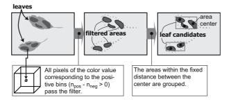
Fig. 2. Process of filtering and detecting candidates
