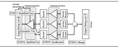
Fig. 1. The architecture of an external sorting algorithm DISTSTRSORT using adaptive construction of a synopsis trie
