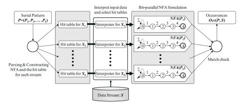
Fig. 2. The framework of our pattern matching algorithm over k-dimension data streams
