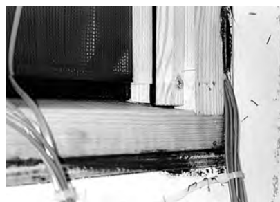
6.9 Mock-up of window integrated solar air collectors on PASSYS test cell, with detail of fabric absorber and air inlet slot
