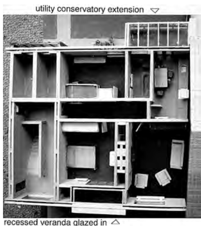
4.8 Plan view of model of passive solar flats at Easthall, with original chimney breast in key location – stacked glazed-in balconies face southeast or west in demonstration
