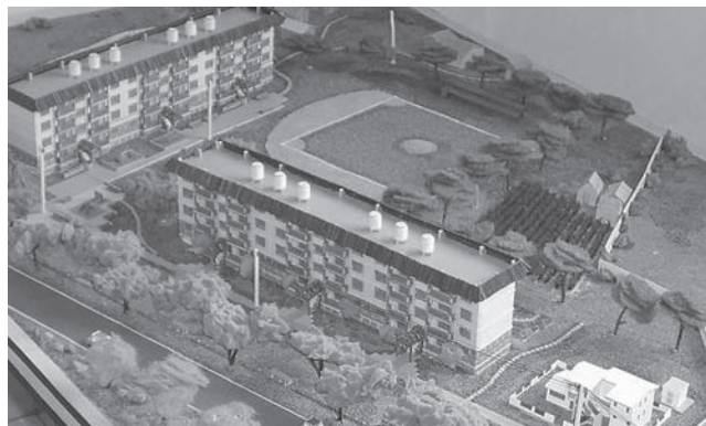
FIGURE 7.5. Architectural model that aims to sustainably enhance the quality of life at a public housing project, El Vallecito, in Pinar del Río Province. The proposal includes adding eaves over windows, planting trees around the complex for beautifying the site and creating more shade, developing more community gardens (right center, to the right of baseball diamond), and rimming the rooftops with a facade to hide cisterns. Courtesy Mabel Matamoros Tuma.
