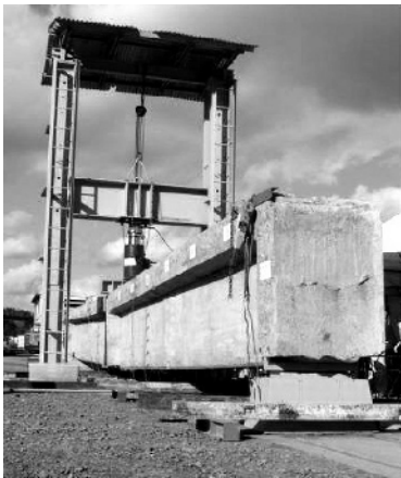
Fig. 13.6. Loading device for a bending test of the girder.
