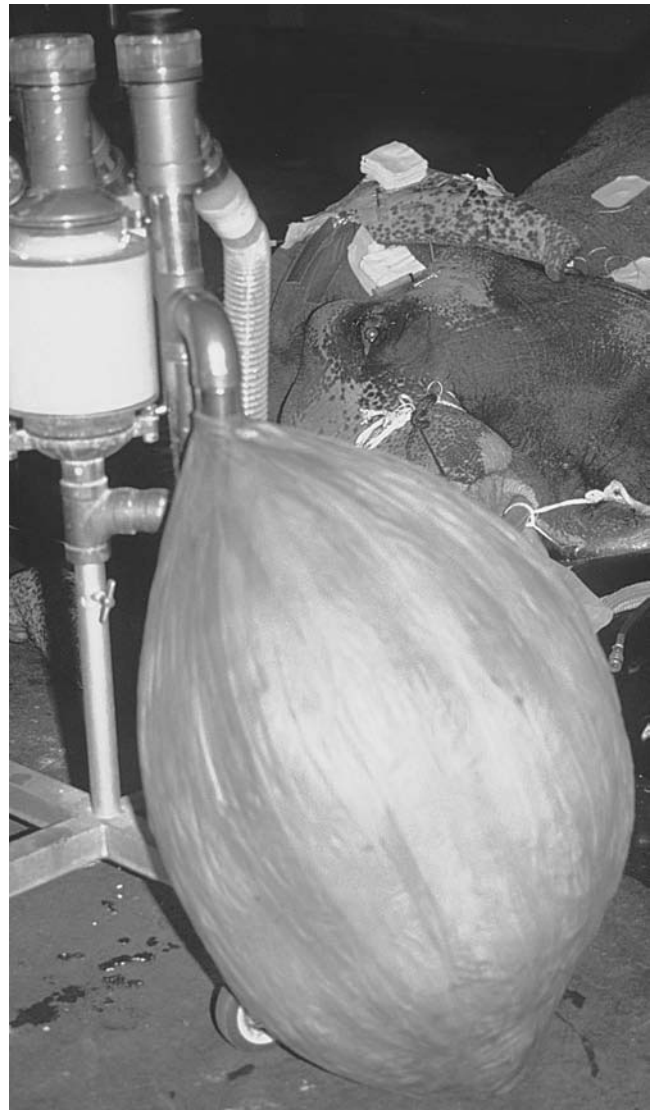
Figure 9.3. A 150 liter weather balloon may be used as a rebreathing bag.
