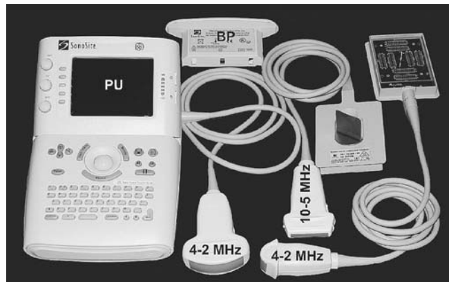
Figure 27.6. Shown is one commercial portable US system (PU), which can be used for elephant assessments. The PU is equipped with one low-frequency (4-2 MHz) convex transducer, one low-frequency (4-2 MHz) micro-convex transducer, and one high-frequency (10-5 MHz) linear transducer.
