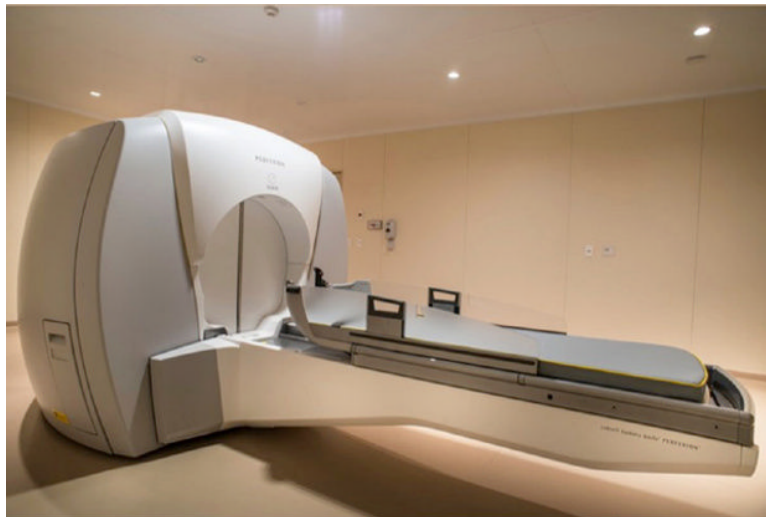
Figure 19.2 Gamma Knife Perfexion® last model installed in the HCor (Hospital do Coração) neuroscience in Sao Paulo, Brazil. This model can be called ‘Plus’ with the addition of a cone beam computed tomography at the entrance of the device to check the patient’s position and target. ( See insert for colour representation of the figure. )
