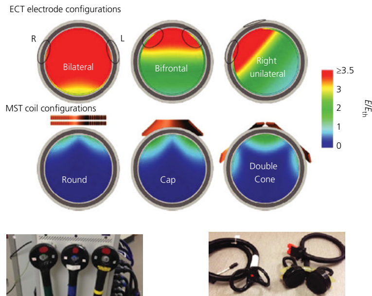
Figure 9.5 Finite element modelling of electric field strength induced in a five-concentric spherical model of the head by ECT (top row) and MST (bottom row) configurations. Adapted from Deng et al. [9]. Photo insert on left shows MagStim Theta Round coil switcher box allowing rapid coil swapping between trains. Photo insert on right shows Magstim Double Cone coil for MST on left and MagVenture Twin-Coil on right. Both deliver a field distribution similar to the double-cone configuration.
