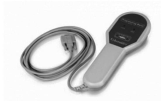
Figure 17.3 Hand-held programming wand transmits information between the VNS programming computer and the VNS pulse generator. Source: Adapted from VNS therapy physician's manual, with permission from Cyberonics, Inc. [27].
