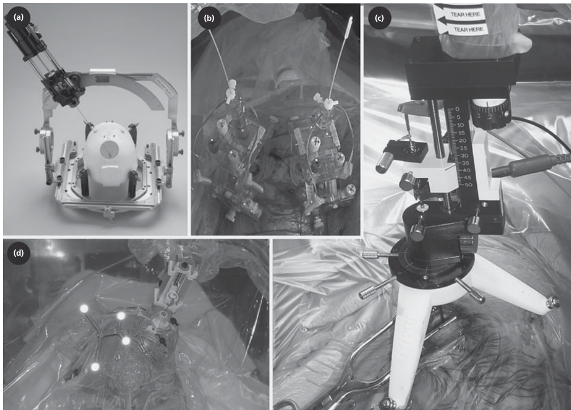
Figure 13.4 Classic and modern stereotactic devices. Classic frames, such as the CRW ( a , Integra), incorporate the fiducials into the stereotactic device using an attached localizer (see Figure 13.1b) during imaging to relate and transform the brain imaging (MRI, CT) space to the physical frame space. The relationship, yielding frame coordinates for adjusting the instrument holder (stereotactic arc, as shown), is calculated using software or by direct measurement on X-ray, CT and/or MRI. Newer stereotactic devices use different approaches. The microTargeting platform ( c , Fred Haer Corp.) physically separates the imaging fiducials from the frame. The fiducials are physically attached to the patient's head before CT and MRI imaging and the trajectory is planned on proprietary software. An acrylic stereotactic platform is custom-manufactured (white tripod in c ) that attaches to the fiducials, instantiating in physical space the imaging-planned trajectory (the picture shows the microelectrode drive attached to the platform). The NexFrame ( d , Medtronic) also separates the fiducials from the frame. A CT is performed with fiducials attached and co-registered to an MRI for trajectory planning. In the operating room, the relationship of the imaging fiducials to the NexFrame, a plastic stereotactic device affixed atop the burr hole, is calculated by software after detection of their location in physical space using a camera to visualize reflective balls (seen in picture attached to the stereotactic device). The Clearpoint Smartframe ( b , MRI Interventions) utilizes a fiducial cannula prefilled with gadolinium. The stereotactic device is affixed to the patient in the MRI scanner, and the relationship of the cannula (physical space) to the brain space is determined with an MRI. The software calculates the necessary adjustments to align the attached tower containing the fiducial cannula to the planned trajectory, which are made using four coloured knobs. The DBS is inserted through the fiducial cannula, as shown. ( See insert for colour representation of the figure. )
