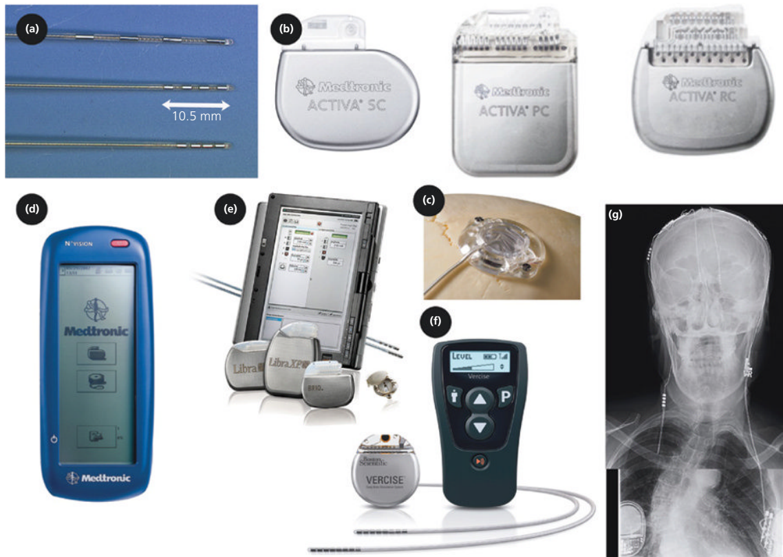
Figure 13.2 Deep brain stimulation equipment. (a) DBS leads of different configurations. The contacts of the bottom two leads are 1.5 mm long cylinders, separated by 1.5 mm (middle lead) or 0.5 mm (bottom lead). The upper electrode array has larger contacts (3.0 mm) and wider spacing (3.0 mm) adapted for use in the anterior internal capsule (e.g. for OCD; in the United States, this is the only use for which this lead is approved by the FDA, under a HDE). (b) Internal pulse generators (IPGs) are primary cell (left and middle) or rechargeable (right), and either single channel (left) or dual-channel (middle, right). (c) StimLoc ring for anchoring the DBS lead to the bone and covering the burr hole. (d) IPGs are programmed telemetrically. Source: a–d reproduced with permission of Medtronic. (e) St. Jude Medical also offers single (left) and dual-channel (centre, right) IPGs, as well as a dual-channel rechargeable IPG (right); depicted also are the DBS electrodes, and the burr-hole anchoring device. Source: Reproduced with permission of St. Jude Medical. (f) Boston Scientific offers a dual-channel rechargeable IPG, and DBS leads with eight closely spaced contacts. Source: Reproduced with permission of Roshini Jain. (g) X-ray showing bilateral DBS leads, extension cables connected in the head (left side of figure) and neck (right side of figure), and IPGs. In fact, the latter is a poor location for the DBS-to-extension connection to be located, which predisposes to breakage, which occurred with a previous right extension cable where the connection was in the neck (left side of figure).
