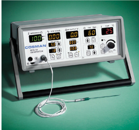
Figure 21.1 A modern RF generator. The Cosman RFG-1A generator is shown, which includes real-time impedance and temperature monitoring, stimulation capability, automatic temperature control and freehand output control capability. Also shown is a lesioning electrode with built-in thermocouple. Source: Cosman Medical, Inc.
