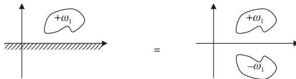
FIGURE 6.14 Illustration of the method of images for the flow near a horizontal wall generated by a vorticity distribution. An image distribution of equal strength and opposite sign mimics the effect of the solid wall.
