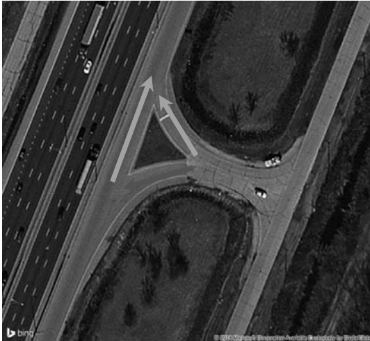
Fig. 1. Button-hook ramp connected to parallel frontage road with proper (green) and wrong (red) movements.
