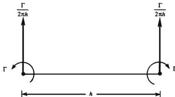
FIGURE 5.14 Interaction of line vortices of opposite spin, but of the same magnitude. Here \Gamma refers to the magnitude of circulation, and the induced velocities are in same direction and perpendicular to the line connecting the vortices. Thus, if free to move, the two vortices will travel along straight lines in the direction shown at speed \Gamma/2\pi h .
