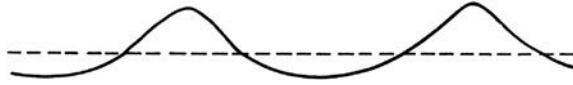
FIGURE 8.22 The waveform of a Stokes wave. Stokes waves are finite-amplitude, periodic irrotational waves in deep water with crests that are more pointed and troughs that are broader than sinusoidal waves.
