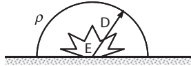
FIGURE 1.12 In an atmosphere with undisturbed density \rho , a point release of energy E produces a hemispherical blast wave that travels a distance D in time t .
