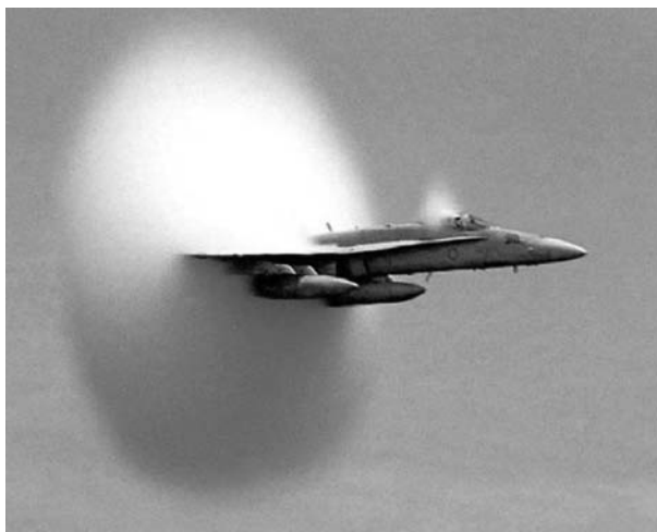
Fig. 12.3 An F/A-18 Hornet as it breaks the sound barrier. (Ensign John Gay, USS Constellation , U.S. Navy.)
