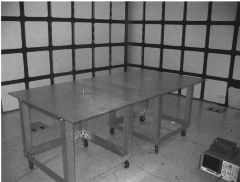
Figure 4.3 Monopoles mounted on ground plane situated in anechoic chamber.
