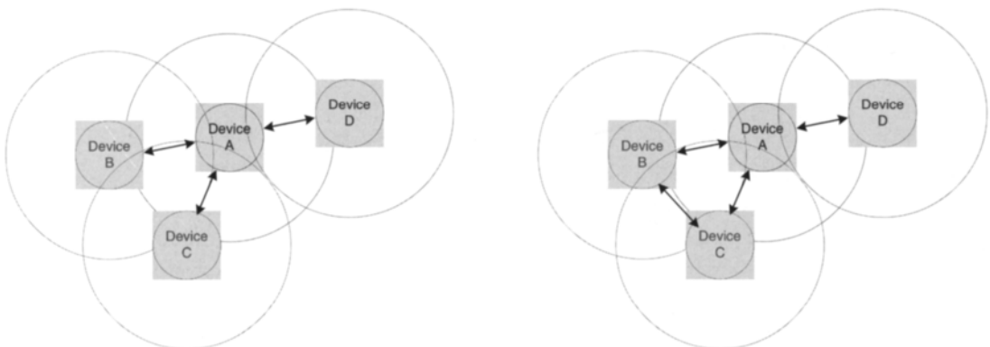
Figure 9.3 Central and distributed arrangements.
