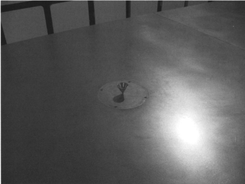
Figure 4.2 Conical monopole mounted on large ground plane.
