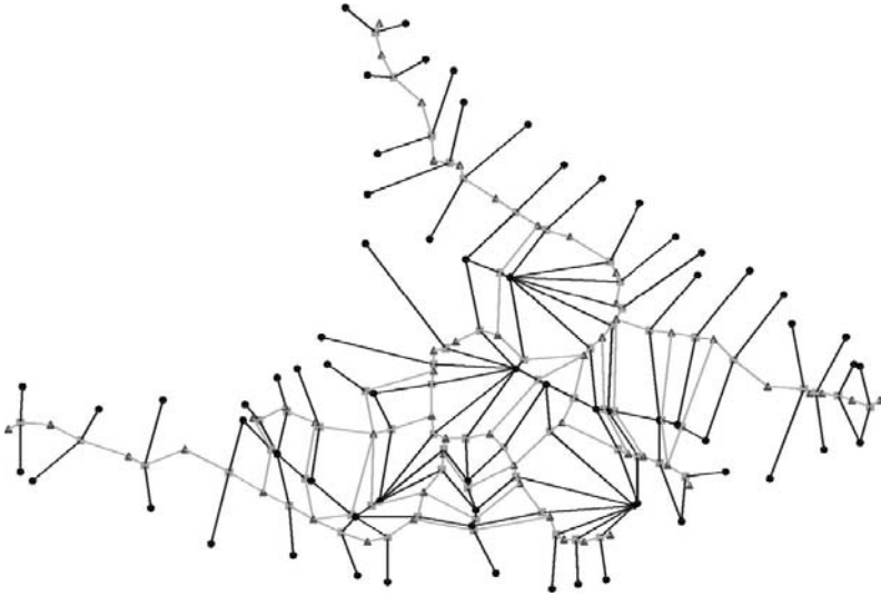
Figure 2.5 Pfaltz graph corresponding to a topographic surface situated in the Latschur Mountains, Austria. Legend: circles – pits, triangles – peaks, squares – passes
