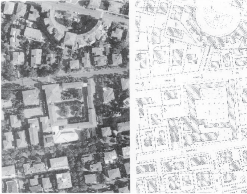
Figure 4.12 Example of aerial photos and the corresponding data in the database. The goal is to compare the map and the photos in order to find the differences and to update automatically the database (Tellez and Servigne 1998).
