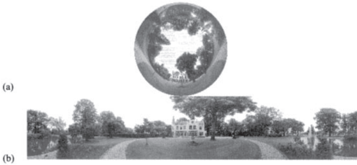
Figure 3.14 Example of a fish-eye photo and its transformation, (a) Cycloramas are digital panoramic images with a horizontal field of view of 360° and a vertical field of view from 30° below up to 60° above the horizon. (b) CycloMedia is the brand name of the Frank Data products on the market.
