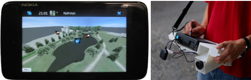
Fig. 1. Two HYDROSYS mixed reality platforms. (left) A cell phone for augmented virtuality. (right) An ultramobile PC equipped with orientation sensors and camera for augmented reality.
