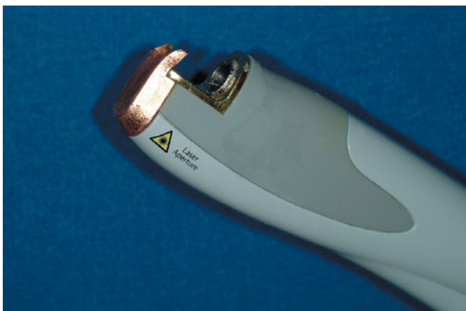
Figure 10.5 Laser hand piece. A cooling plate that is a fixed part of the laser hand piece is recommended
