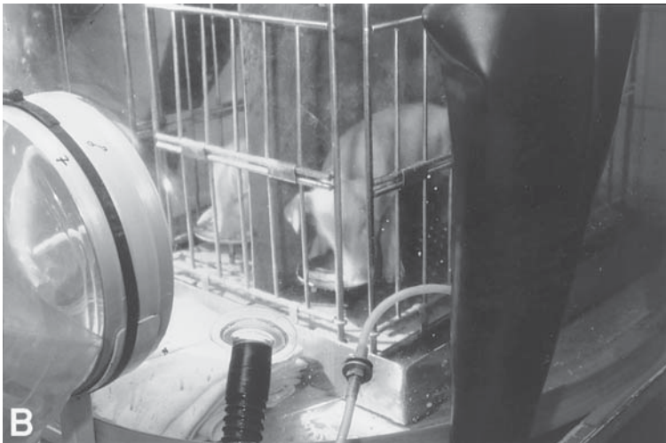
Fig. 5. (A) Peristaltic milk pumps on the floor of the animal laboratory. They are connected to the milk bags underneath the isolators. (B) Feeding of the piglets. Connections from left to right: PVC tunnel, air duct, milk duct.
