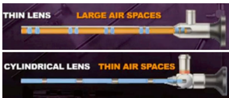
Fig. 9.3 Optical principles of modern hysteroscopic technique
