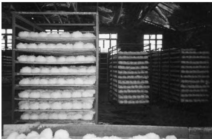
FIGURE 17.5 (Color figure follows p. 232.) Resembling a bakery, this is the oven/hot air chamber where the Tremella fuciformis fruiting bodies are placed for drying.
