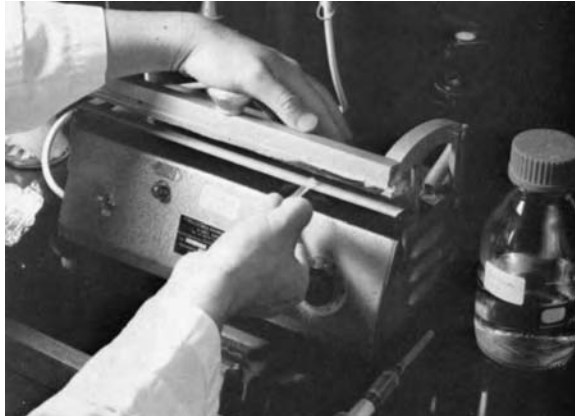
FIGURE 10.5 Sealing the end of a short drinking straw with a polythene heat-sealer.
