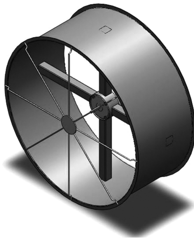
Figure 6.7 Exhaust Fan – CAD.
