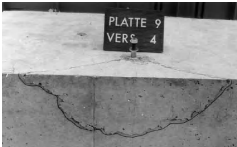
Fig. 4.72 Concrete edge failure of a shear-loaded anchor close to an edge (taken from Fuchs, Eligehausen (1986))
