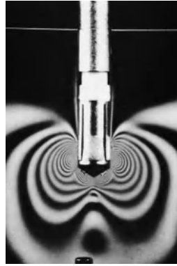
Fig. 2.22 Stress contours in the anchorage zone of a torque-controlled expansion anchor (Seghezzi (1983))
