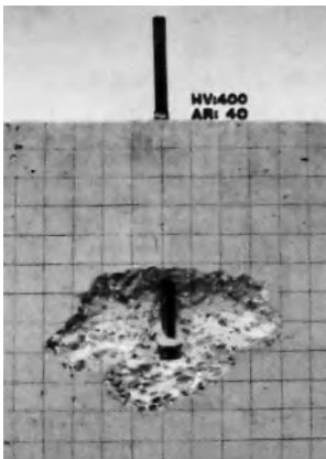
Fig. 4.44 Local side blow-out failure of a headed stud loaded in tension with small edge distance (Furche, Eligehausen (1991))
