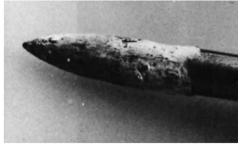
Fig. 8.6 Photo of a power actuated fastener after a tension test in cracked concrete (taken from Eligehausen (1988/2))
