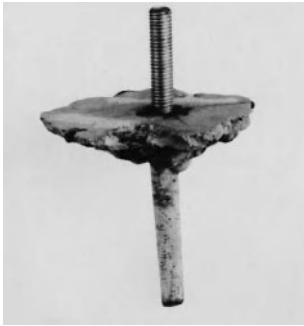
Fig. 6.2 Photo of a bonded anchor after tension test (Eligehausen, Mallée, Rehm (1984))
