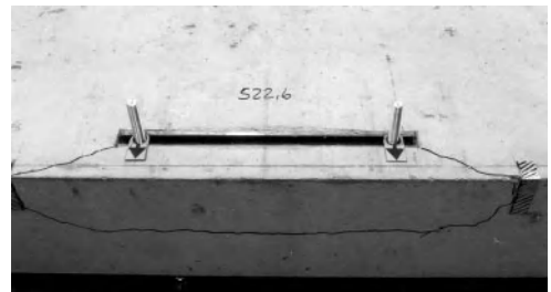
Fig. 5.15 Photo of an anchor channel after test; concrete edge failure. Spacing of anchors equal to 5 times the edge distance ( Forschungs- und Materialprüfungsanstalt Baden-Württemberg (1995/2))
