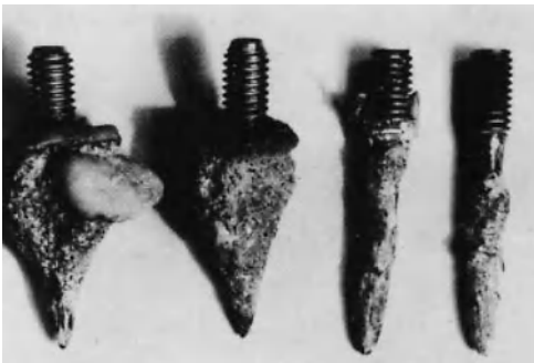
Fig. 8.1 Pulled out power actuated fastener (Patzak (1979))
