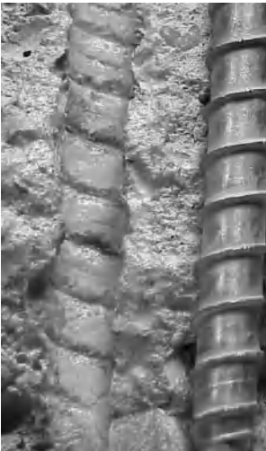
Fig. 9.1 Screw anchor and a thread cut into the wall of the drilled hole (Küenzlen, Sippel (2001))
