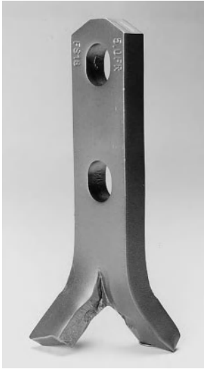
Fig. 2.5 Steel flatbar with "fishtail"
