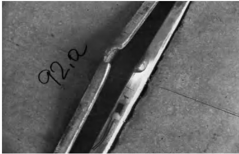
Fig. 5.3 Photo of an anchor channel after test; failure by distortion of anchor flanges (Wohlfahrt (1996))
