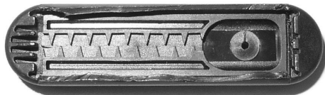
Figure 5 Typical plastic injection molding variables: a single part with 42 critical dimensions.
