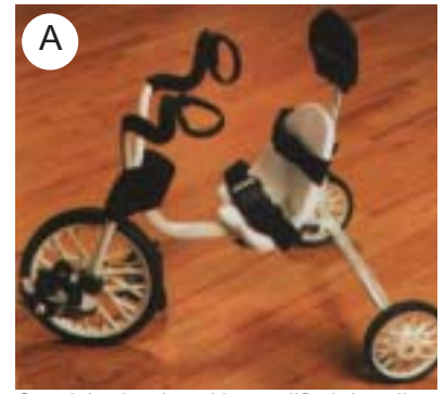
Special tricycle with modified handles, head rest and restraints for the body.
