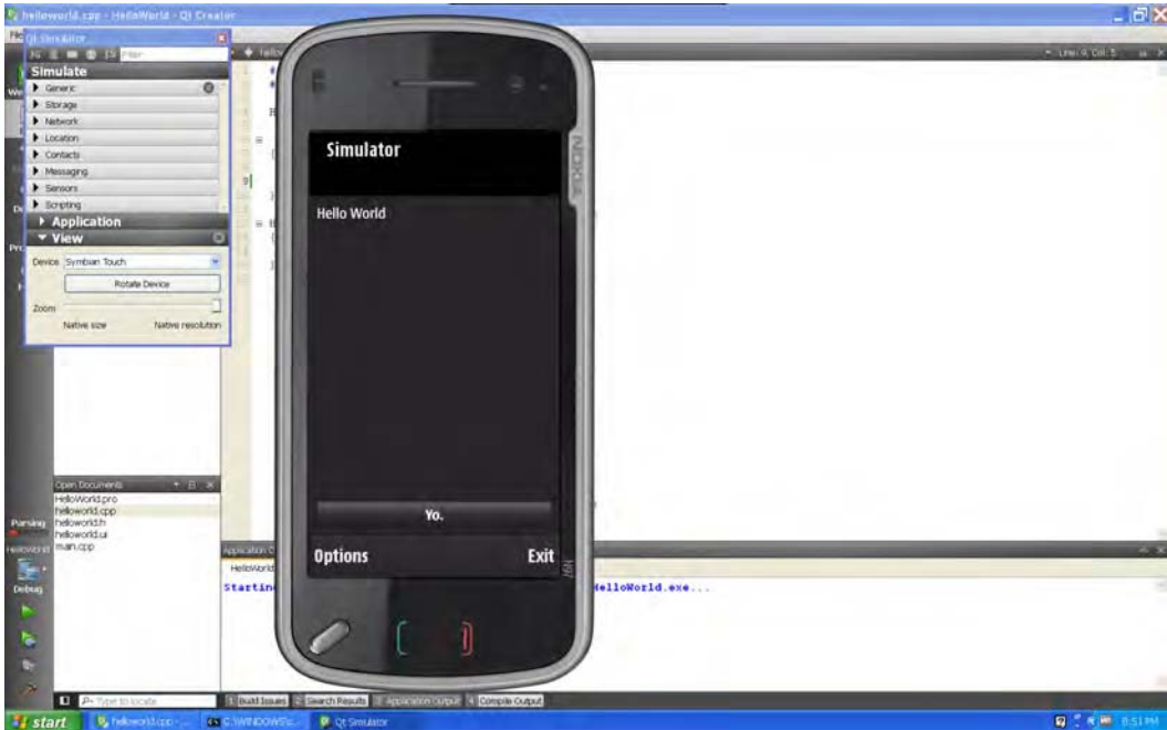
Figure 3–8. Hello World, compiled and running in the Qt Simulator.
