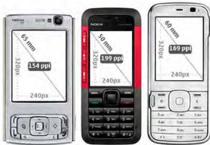
Figure 2–9. These three devices have the same resolution, but different physical screen sizes (courtesy Forum Nokia)
