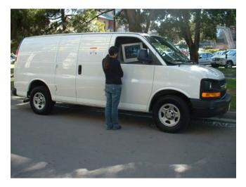
**Fig. 1.** SVEN in its van configuration—aka *SVAN*. A camera with telephoto lens is mounted on the front of the SVAN roof and points at unsuspecting pedestrians up to 150 meters away. The monitor in the window displays video to other pedestrians as they pass the van. Speakers just inside the van window play corresponding music when the system is generating a music video.
