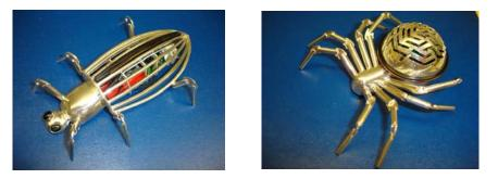
**Fig. 5.** The photographs shows a Bombardier Beetle brooch including inbuilt scent dispenser, and Spider brooch with inbuilt humidity sensor, which measures the humidity of the user's breath as a message is whispered into the abdomen. Photograph by Gareth Jenkins.
