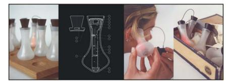
**Fig. 2.** "Message in a Bottle", each bottle contains a small electronic circuit which can capture a telephone message (via RF) or an audio message from the user (via hidden microphone inside). A small diode light array inside each bottle provides feedback whether a message is stored, recorded or played back.
