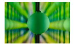
Fig. 4. Close-up of a NOVA voxel. The diameter of each voxel is 40mm and each voxel contains control electronics and 12 LEDs for full-color RGB.
