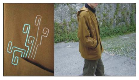
Fig. 4. the Compass Coat; on the left a detail of the Electroluminescent wire on the pocket
