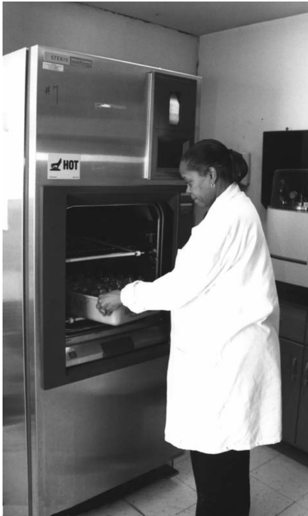
Figure 3.3 A typical steam autoclave for sterilizing small laboratory and surgical items, microbiological media, and other materials that can withstand the effects of 20 to 30 min in saturated steam at 121°C.
