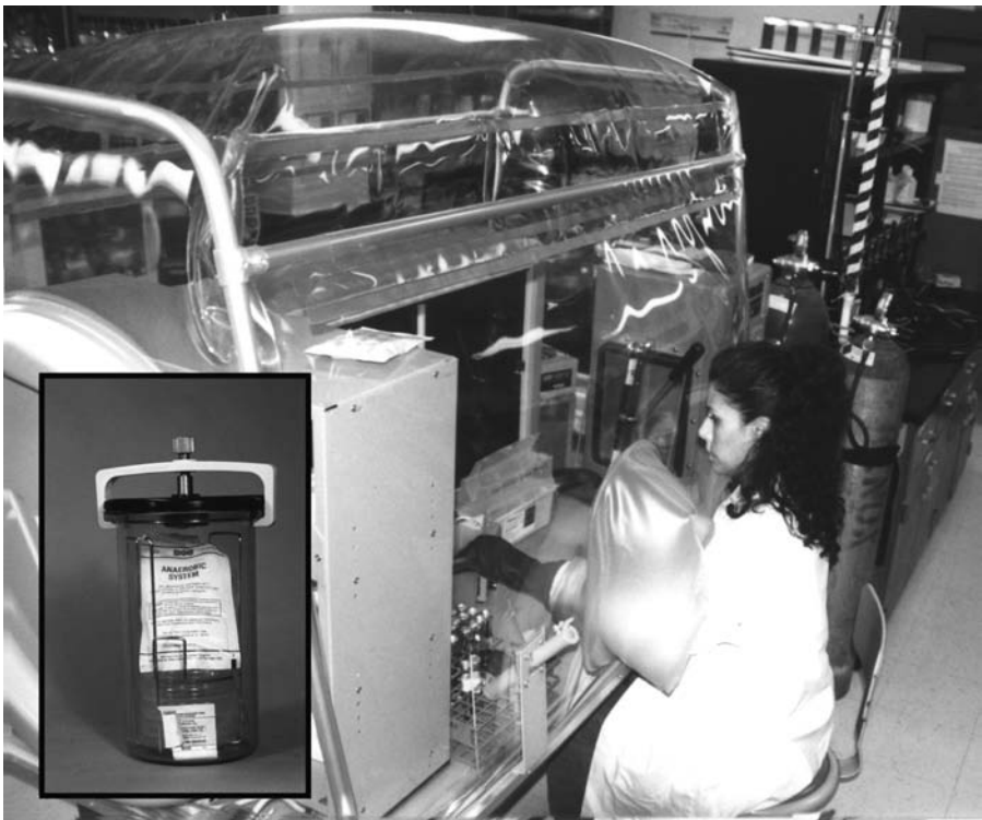
Figure 2.5 Anaerobic chamber for handling strict anaerobic bacteria. All manipulations, including inoculations and incubation, are carried out in a oxygen-free atmosphere. Insert: An anaerobic jar.
