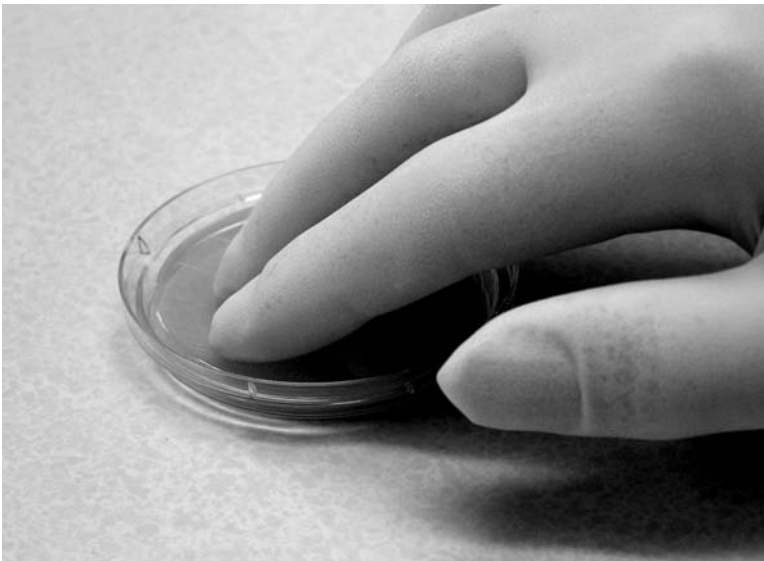
Figure 5.9 Gentle pressure is applied to a RODAC plate when sampling a flat surface.
