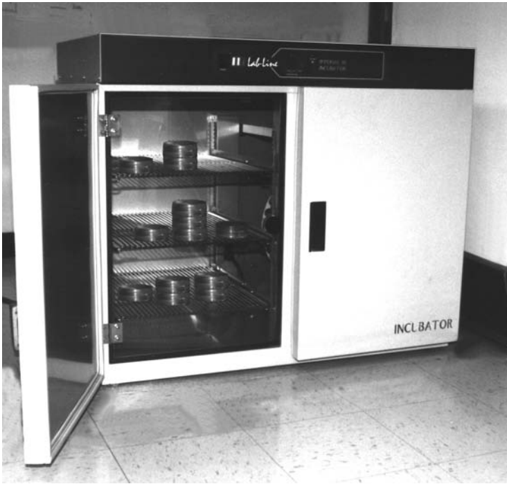
Figure 2.4 A microbiological incubator. Thermostatically controlled chamber can be maintained at a constant temperature appropriate for the species to be grown.
