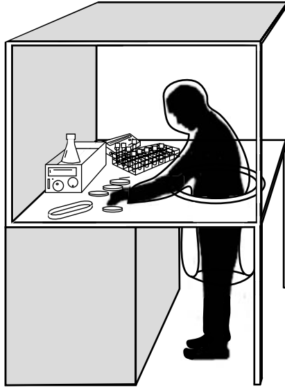
Figure 4.8 Basic concept of a half suit isolator. Technician conducts sterility tests within a sterile isolator chamber while completely enclosed in an airtight suit. The suit is entered from below. Isolator normally would have several ports or air locks to transfer materials aseptically in and out of the chamber.
