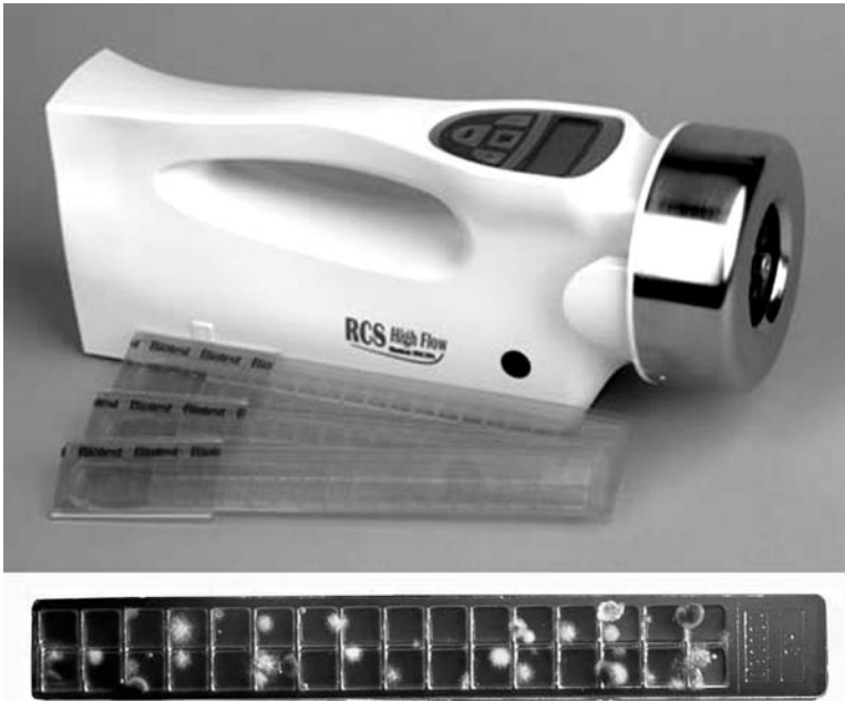
Figure 5.4 An RCS centrifugal air sampler, with three sample strips. Below, a sample strip following incubation. (Photo courtesy Biotest/Carol Julich.)
