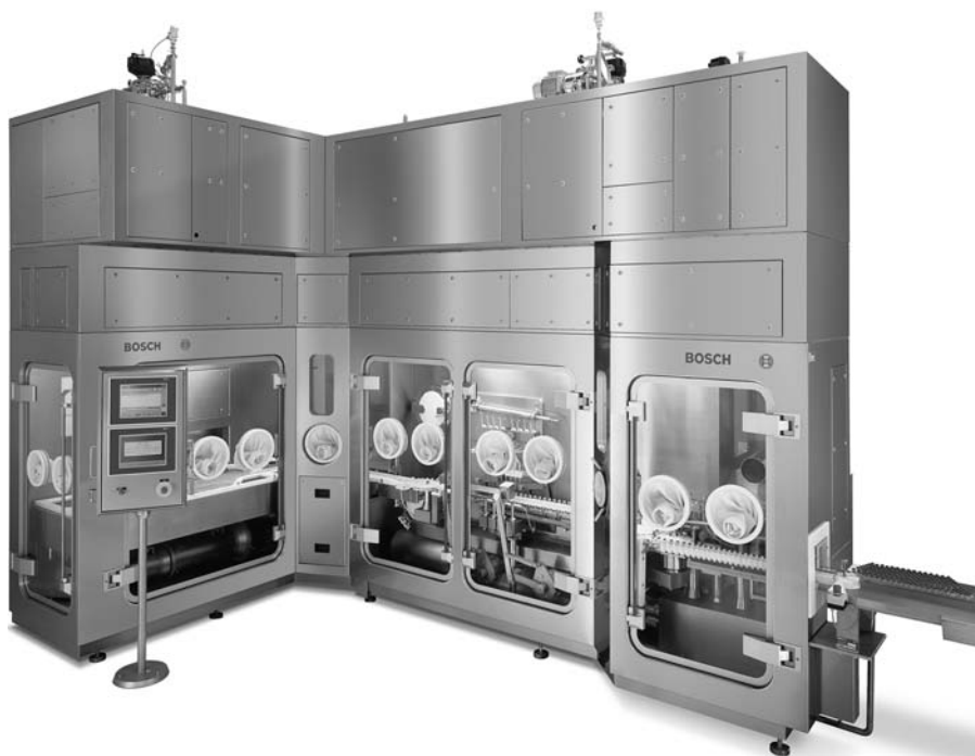
Figure 4.7 An isolator enclosing an aseptic filler. Numerous glove ports provide sterile access to machinery when necessary. (Photo courtesy Bosch Packaging Technology/John L. Kirk.)
