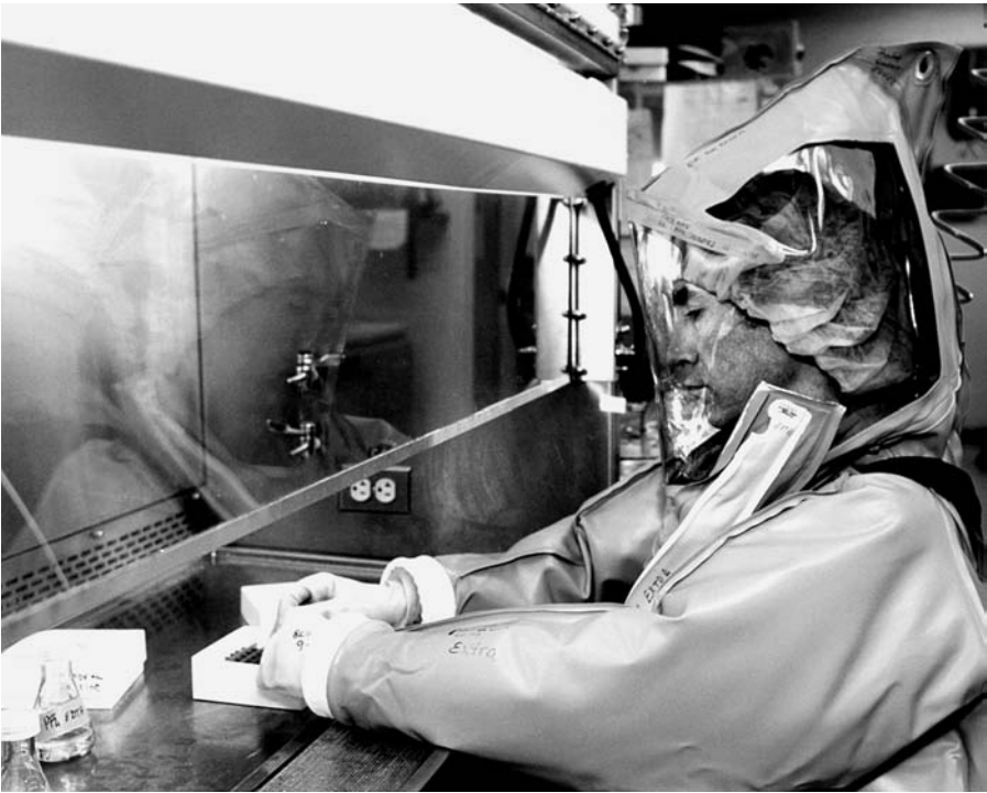
Figure 4.10 A BSL4 laboratory. Technician wearing a positive pressure suit while working at a Class II BSC. Breathing air is supplied by coiled air hose behind worker's head. (Photo: CDC Public Health Image Library ID #1860.)
