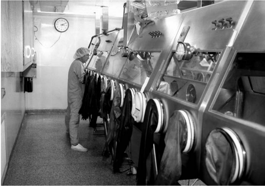
Figure 4.6 Class III biological safety cabinets. (Photo: CDC Public Health Image Library ID #2548.)
