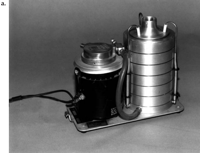
Figure 5.1 (a) Andersen six-stage sieve sampler. Cross section (b) shows typical pathway of air as it passes through successive perforated stages of decreasing hole size and increasing stream velocity. Captured particles are sorted according to size. See Table 5.1. Continued.
