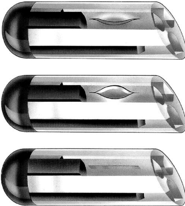
Figure 4.11 (a) Magnified image of the valve near the tip of a triple lumen Groshong catheter (Bard USA). Aspiration of the lumen induces a negative pressure opening the slit valve inwards (upper image). Flushing the device induces a positive pressure opening the slit valve outwards (middle image).
