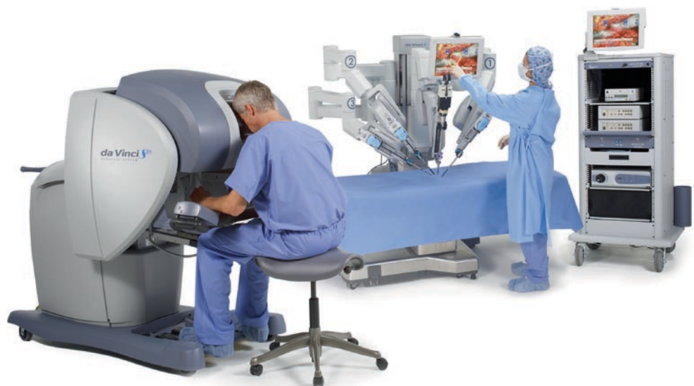
Fig. 1.1 The da Vinci S surgical system. The three components are shown: the surgeon console, the 4-armed surgical robot, and the endoscopic stack. Courtesy Intuitive Surgical, CA
