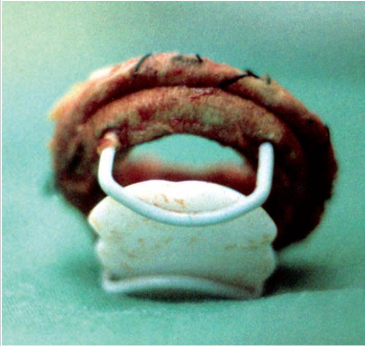
**Fig. 9.3** Disc valve Beall explanted due to structural dysfunction 16 years after implantation. Uneven wearing of the disc
