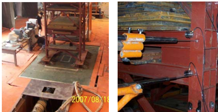
Figure1 earthquake pedestal and detection equipment
