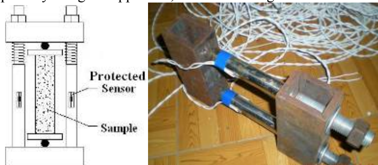
Figure 1. Specially designed apparatus for preloading
