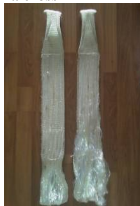
Figure 6. Failure pattern of polyester belt
