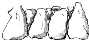
Figure 4.2. Packing wedges, drawing by Rabia Charef-Morel from [GUI 08]
