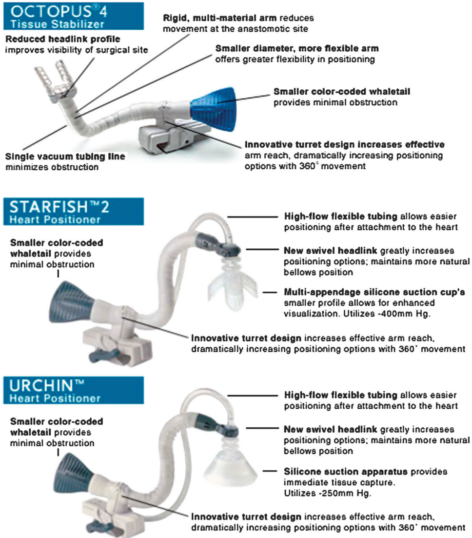
Figure 14.7. OPCAB tissue stabilizers: the Medtronic Octopus 4, Starfish 2, and Urchin. From www.medtronic.com .
