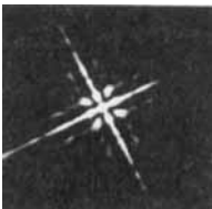
Fig. 6. The diffraction pattern obtained by shining a fine beam of visible light through a fine mesh.
