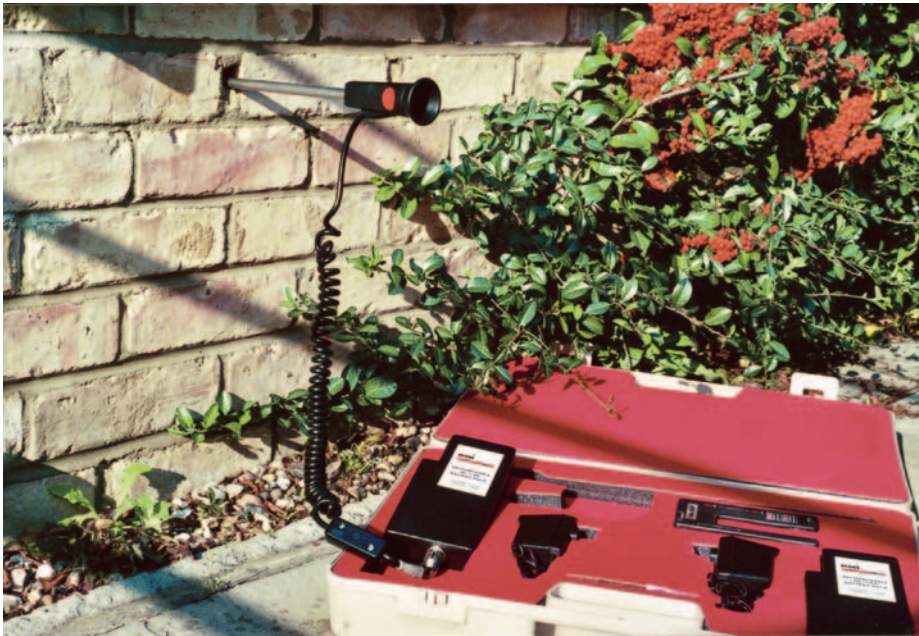
FIG 1.2 Borescope for inspecting inside wall cavities, sub-floor voids and other areas. The wide-angle lens provides good depth of field.
