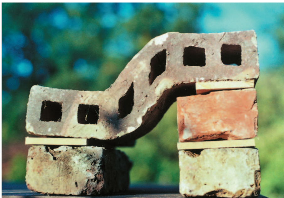
FIG 4.6 The Victorians used special-shaped bricks as wall ties in their cavity walls.
