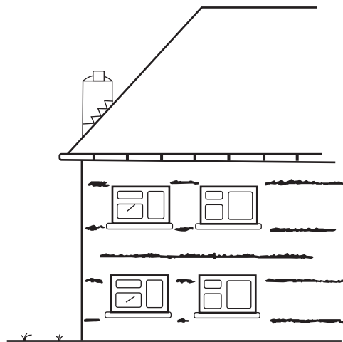
Rusting wall ties
