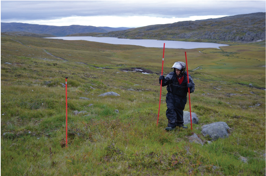
Figure 9.6 The Mining Director marks the locations of the planned drill holes with vertical road sticks
