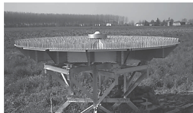
Figure 9.7.23 GNSS receiving antenna with large impedance ground plane.
