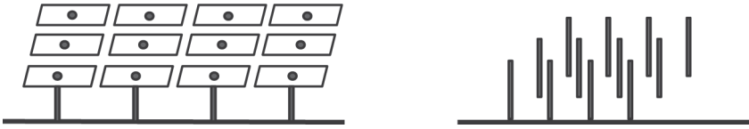
Figure 9.7.14 Impedance structures of mushrooms and straight pins.
