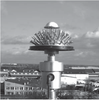
Figure 9.7.33 PN-A5 antenna installed at rotational robot.
