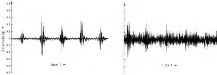
Figure 3. Time record showing a typical fault signature of a defect roller bearing without (left) and with cavitation interference (right)
