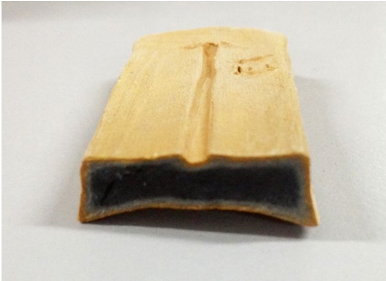
Fig. 21.5 Black core defect in Sabak Bernam clay
