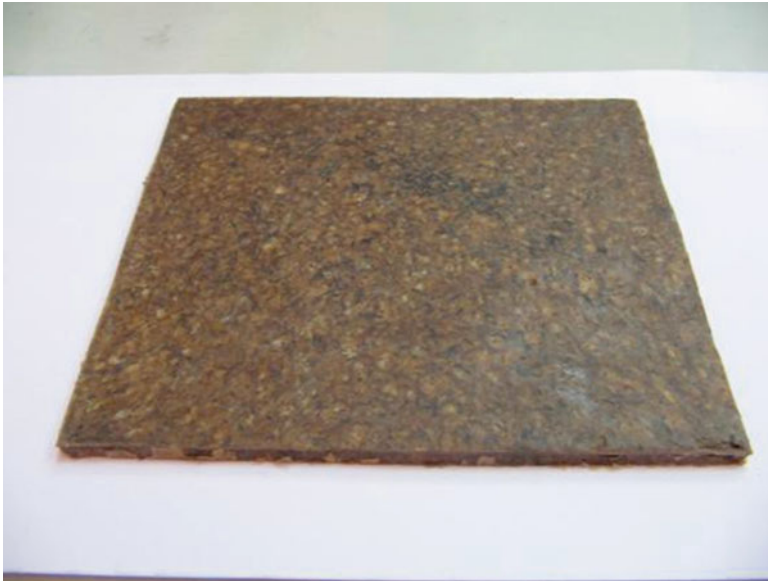
Fig. 48.2 Prototype of synthetic material from sugarcane bagasse as alternative relief print block
