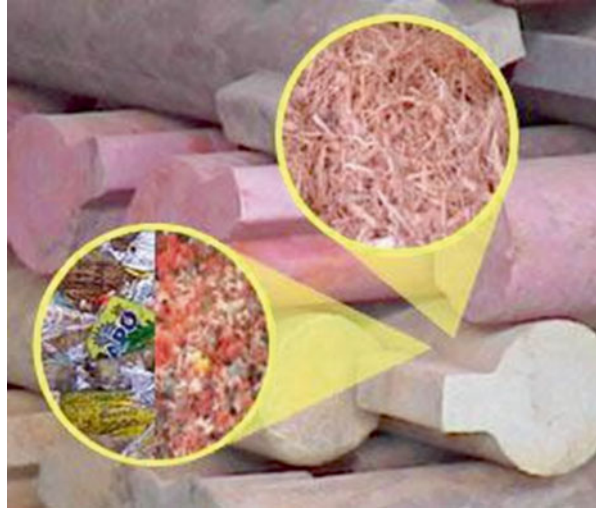
Fig. 48.1 The product of wood plastic composite – sugarcane fiber (Illustration taken from http://www.edraecosisternas.com )
