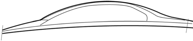
Fig. 29.4 The side-shoulder, also known as the “catwalk,” carries semantic and syntactic functionality as part of the Volvo form language [15, 16]
