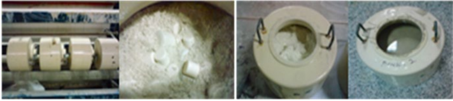
Fig. 32.1 Porcelain milling process by jar mill
