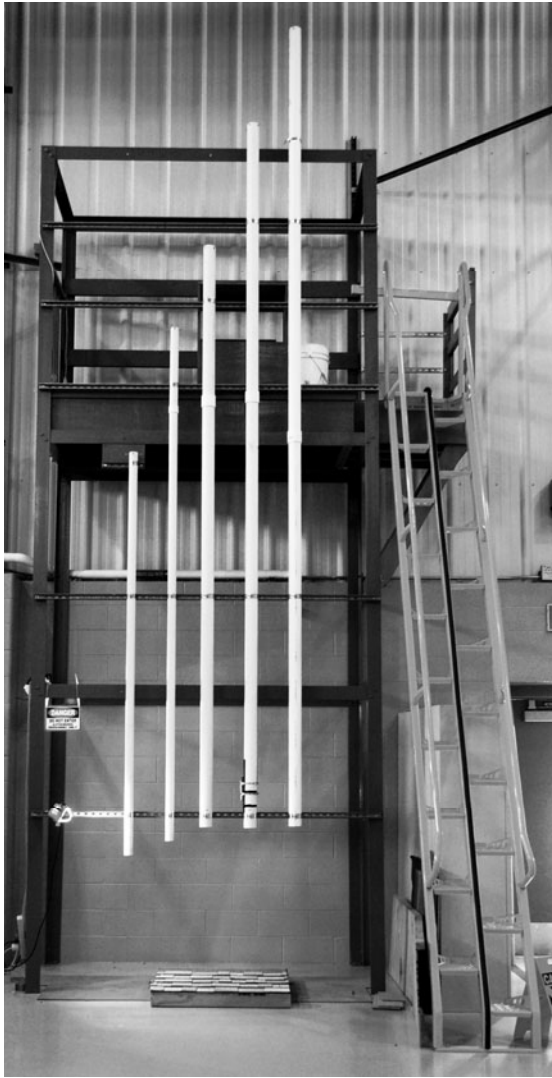
Figure 10.6. UL 2218 Drop Tower
