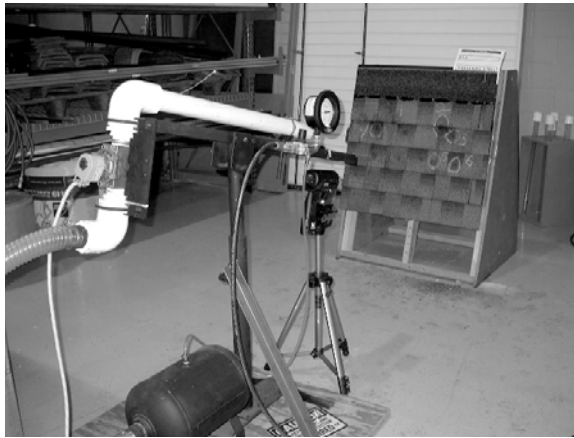
Figure 10.9. FM 4473 Ice Ball Launcher Set-up
