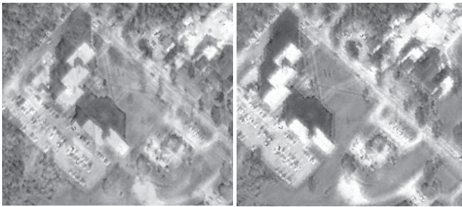
Fig. 8 Influence of overall horizontal parallaxes for effective colour 3D viewing. Left: larger overall horizontal parallaxes may cause stereo fusion problems; Right: small overall horizontal parallaxes are more comfortable for colour 3D viewing.
