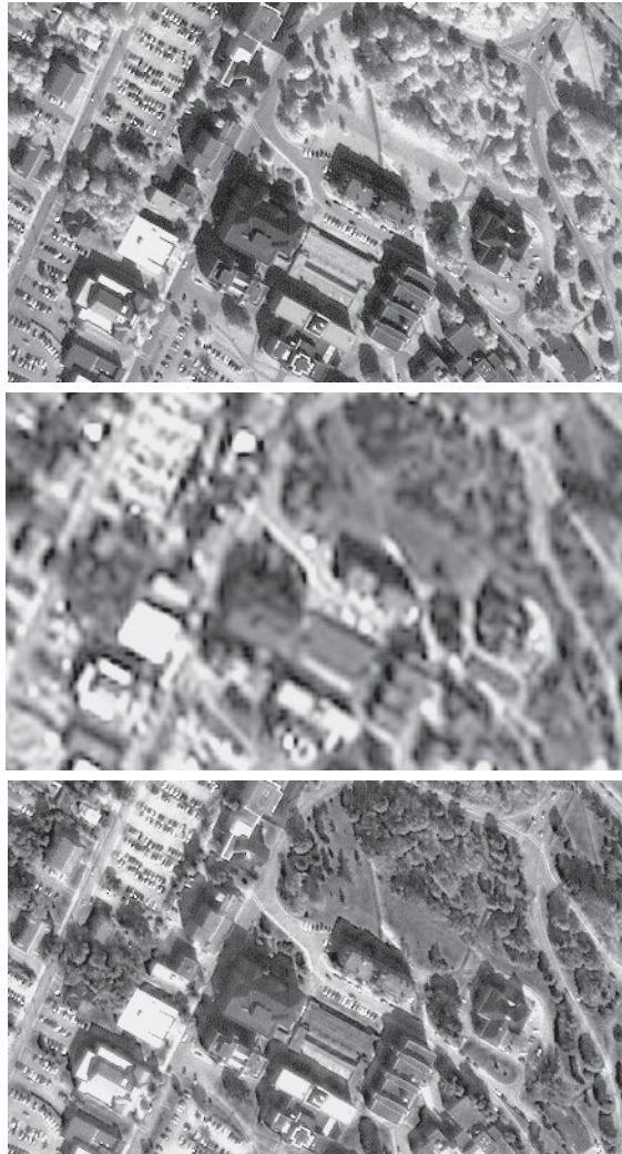
Fig. 2 Automatic image fusion, Ikonos, University of New Brunswick, Canada. Top: Original panchromatic image (1 m); Middle: Original natural colour image (4 m); Bottom: Fused natural colour image (1 m).
