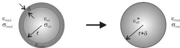
Fig. 7 Single-shell model. Combination of the electrical properties of the membrane and cytoplasm into one effective complex permittivity; \sigma_{med} and \epsilon_{med} are the conductivity and permittivity of the medium, respectively; \sigma_{int} and \epsilon_{int} are the conductivity and permittivity of the cytoplasm, respectively, \epsilon_{mem} is the permittivity of the membrane, \delta is the membrane thickness, r is the cell radius and \epsilon_{eff}^* is the effective complex permittivity of the cell
