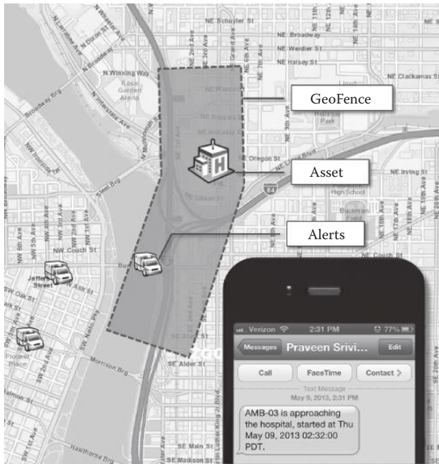
Figure 6.6 Example of Esri’s GeoEvent Processor tool. In this example, an alert is triggered when an ambulance has crossed what is known as a Geo fence or a predefined area of interest that is used to communicate to an asset, which in this example is a hospital. As can be seen in the bottom right of the figure, personnel at the hospital receive an SMS message when the ambulance is arriving. (Copyright © 2014 Esri, ArcGIS, ArcMap. All rights reserved. Used with permission.)
