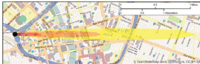
Figure 3.13 A plume generated in ALOHA (top of figure) that is then imported as a KML file into a GIS and layered on a map to show how the plume would affect the area of interest. ALOHA is US government software. For more on using ALOHA with GIS, see http://response.restoration.noaa.gov/aloha and Tomaszewski, Brian. 2003. Emergency response and planning application performs plume modeling. ArcUser , 10–12. (Figure based on map data © OpenStreetMap contributors.)
