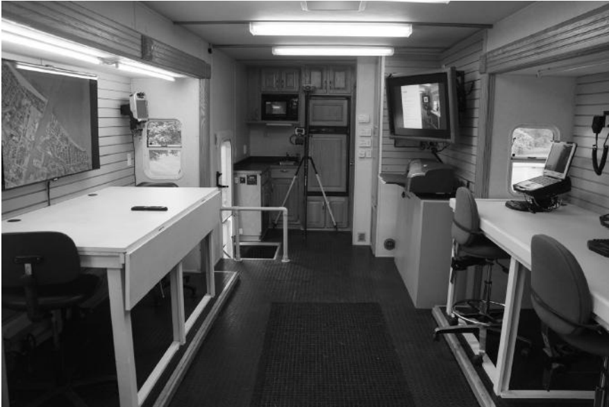
Figure 1.4d View inside the Monroe County GIS technology vehicle looking toward the back. Note work table on the left with a large mapping screen and GPS receiver base station in the rear. (Photo by Brian Tomaszewski. Used with permission from Monroe County GIS.)
