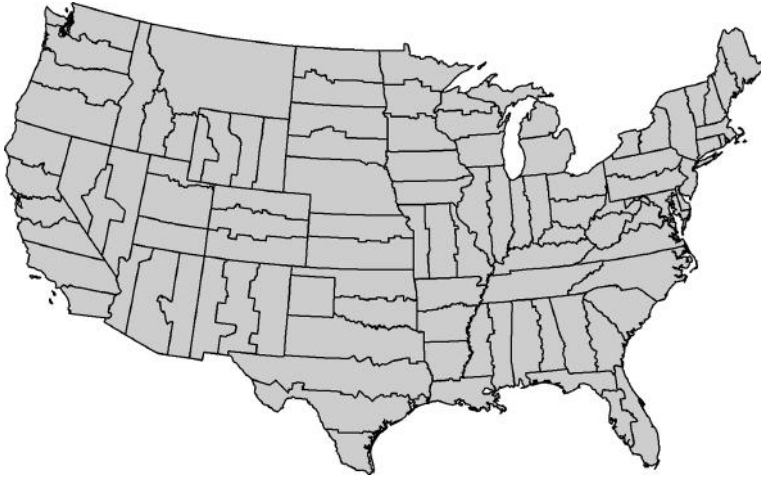
Figure 2.12 State Plane Coordinate (SPCs) zones within the United States. Note that zones do not extend beyond state boundaries and that a state may have several zones. Thus, SPCs are not suitable for regional (i.e., multiple-state) mapping. State plane zones generally measure coordinates in US feet values. (Map by Brian Tomaszewski.)
