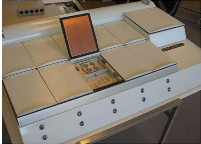
Fig. 1. System of table incubators for single-dish culture. Each chamber has its own lid.
