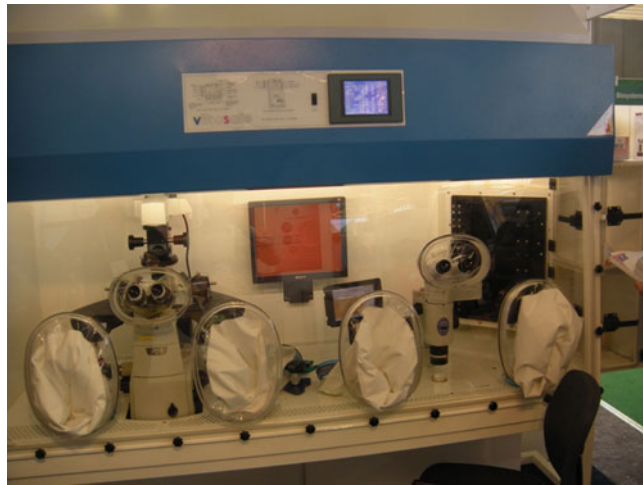
Fig. 2. The incu-workstation has a tightly closed glassy front side with openings for integrated gloves and microscope binoculars. The interior is gassed by \text{CO}_2 and \text{N}_2 and equipped with microscopes. The culture dishes with embryos can remain in the workstation through the whole culturing period.
