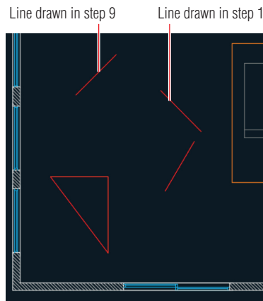
FIGURE 2.18 Angles are relative to the coordinate system in which they are drawn. Both lines were drawn at a 45-degree angle but in different coordinate systems.
