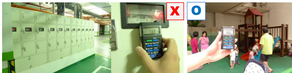
Fig. 19. EMF tests in the electric facility area (left) and the children playground (right)
