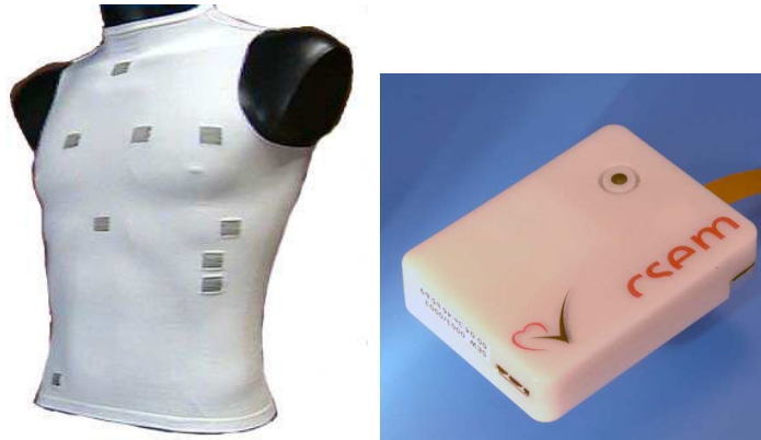
Fig. 5. Inner layer of MyHeart shirt (left) and first prototype of the on-body electronics (right)
