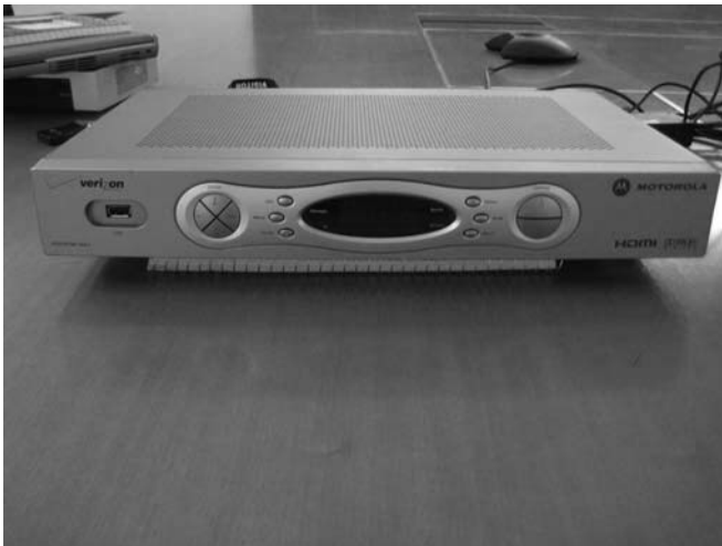
Figure 1.1 An integrated set-top DVR box, in this case supplied by Verizon to its video/DVR subscribers. (Copyright 2009. Property of Verizon. Used with permission. All rights reserved.)
