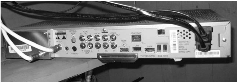
Figure 1.18 Plugs for wires in the back of a DVR set-top manufactured by Motorola, and distributed by cable operator Comcast. (Copyright 2008. Property of Comcast. All rights reserved. Photo used with permission.)
