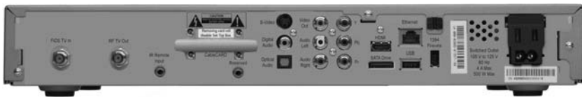
Figure 1.21 Photo of plugs for the wires in the back of a DVR set-top manufactured by Motorola, and distributed by telco operator Verizon. (Copyright 2008. Property of Verizon. All rights reserved. Photo used with permission.)
