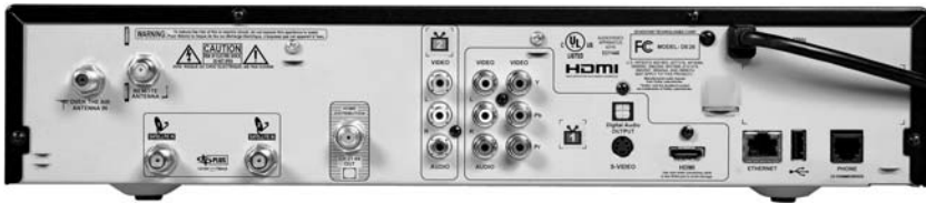
Figure 1.20 Plugs for wires in the back of a DVR set-top manufactured by EchoStar. (Copyright 2008. Property of DISH Network. All rights reserved. Photo used with permission.)
