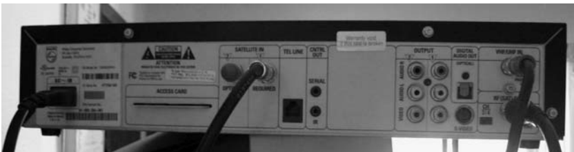
Figure 1.19 Wires in the back of a DVR set-top manufactured by Hughes Network Systems for DirecTV and for TiVo. (Copyright 2008. Property of Willy Schaeffler. All rights reserved. Photo used with permission.)
