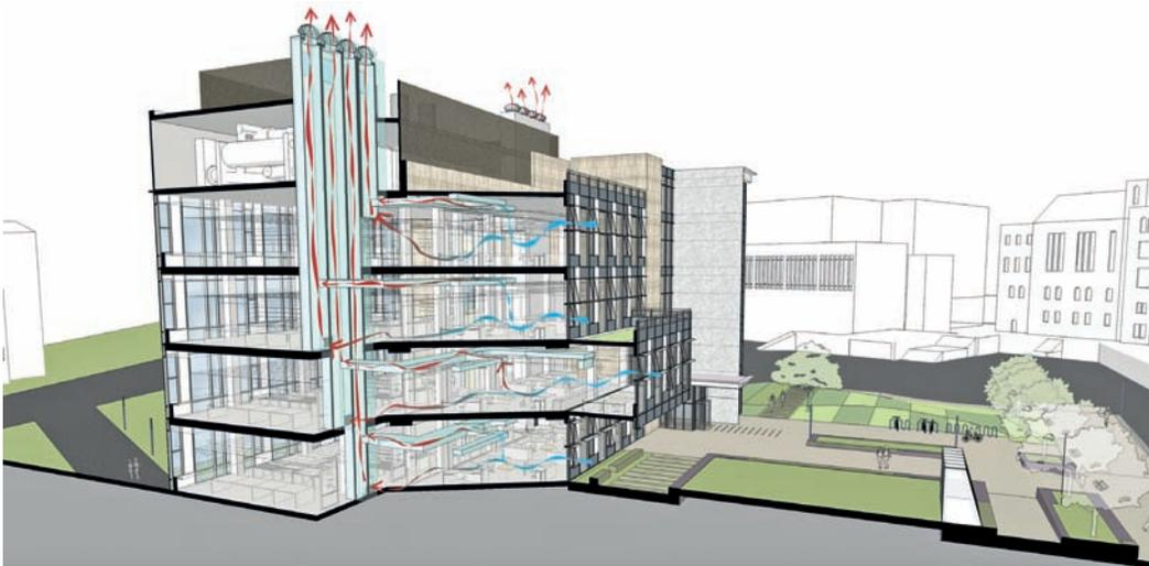
More detailed simulations were not necessary, as the stack exhausts incorporated a number of enhancements to airflow: "solar chimney" windows at the top of the stack super-heat the air which increases the airflow; turbine ventilators, which are driven by wind; and back-up electric motors to drive the turbines in case the airflow is not adequate.
