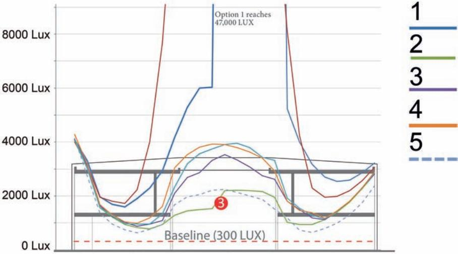
Reflectances were set as: ceiling = 80%, wall = 50%, floor = 20%, and illuminance sensors were placed 30" above the floor.
